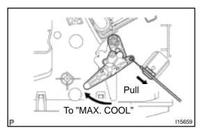
(e) Adjust air mix damper control cable. Set the air mix damper control lever to "MAX. COOL" position and connect the inner cable to lever pin and clamp the outer cable.
